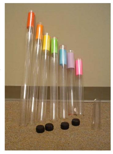
other notes. We put black duct tape over the opening in these caps. This can demonstrate the difference in natural frequencies between "open end" and "closed end" organ pipes of the same length. We taped pieces of colored paper in each tube to make it easy to sort the tubes by note. These colors are used on our PowerPoint music sheets below.
